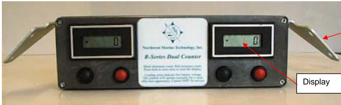
Front View of Dual Counter. Black Switches decrease the count (-). Red Switches increase the count (+).
