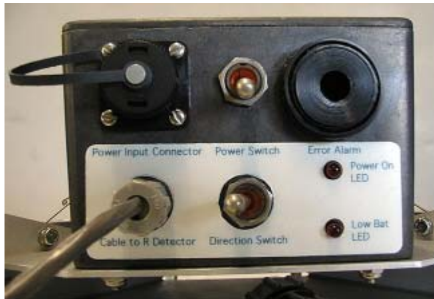
End View of Gate Electronics Box
