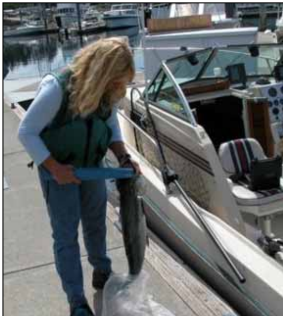
Wands are used in a variety of settings to detect Coded Wire Tags in body locations (top) and in the snouts of salmonids (bottom).
