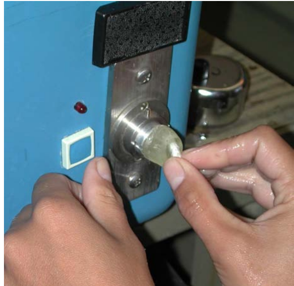
A FWC Biologist implants a full length CWT into the nape musculature of a 30mm SL hatchery red drum, Sciaenops ocellatus using custom made positioning jigs.
